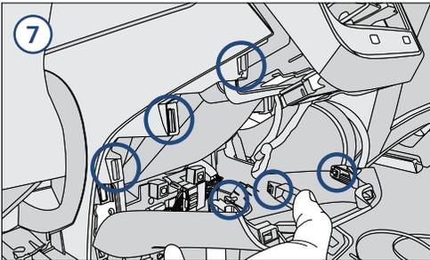
**Step 7** Carefully remove the panel under the air vents by gently pulling on the panel backwards, unclipping the clips.
