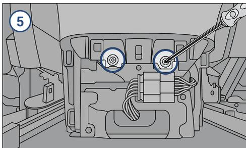
**Step 5** Use a size T20 Torx driver to remove the two screws as shown.
