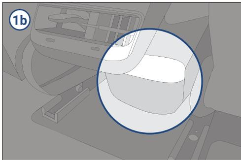
**Step 2** This panel is held in place by five push-fit clips. The clips will release when you apply some force to pull the panel open. Using the trim removal tool provided, slide the end of the tool under the panel on the right-hand side.
