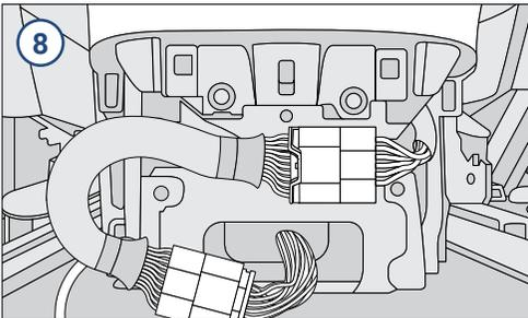
**Step 8** Disconnect the two blue connectors, then plug the T adapter harness in line.
