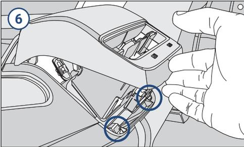
**Step 6** Carefully unclip and remove the air-vent panel.
