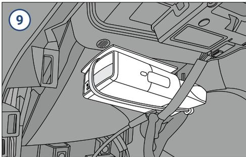
Clean the plastic surface with an alcohol wipe, and wait a few seconds for it to dry.
